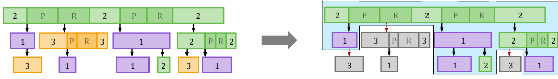
Figure 3.2. (Left) A full busy period tree. Nodes are labeled with their class. Classes 1, 2, and 3 are purple, green, and orange respectively. Overhead is shaded darker. Pause and resumes are labeled with “P” and “R” respectively. Arrows are drawn from jobs to the jobs that arrived during their service. (Right) Highlighting the class < 3 busy period tree with a blue background and black outline. Jobs of class 3 and their descendants are greyed out because they are not included in a class < 3 busy period tree.
